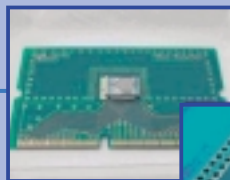
The Point-of-Care chip : integration of DNA sample amplification and analysis by hybridization
