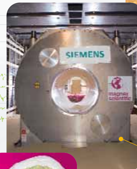
7 TESLA MRI SYSTEM INSTALLED AT NEUROSPIN.
